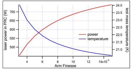
With the full power (825W), we calculate the temperature. With the fixed temperature (20K), we calculate the power.
