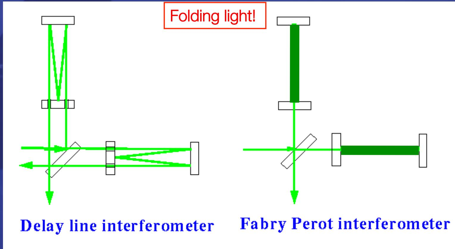
**Delay line interferometer**
