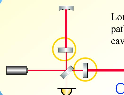
Longer folding light path using Fabry-Perot cavity
