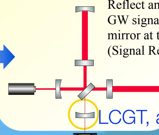
Reflect and enhance the GW signals by additional mirror at the dark port (Signal Recycling, RSE)
