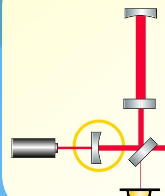
Enhance inside laser power by reflecting coming back light using additional mirror at the laser port
