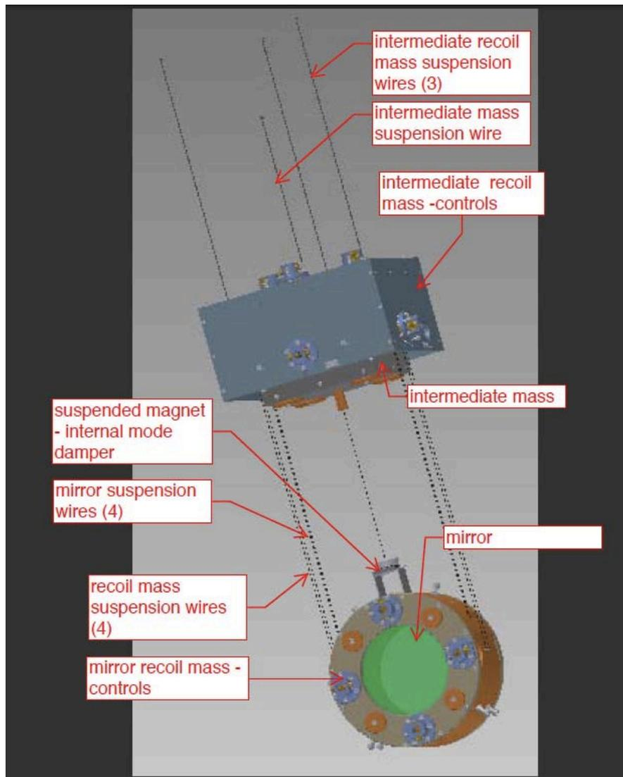
Figure 5: Schematic view of the mirror suspended from the intermediate mass.
