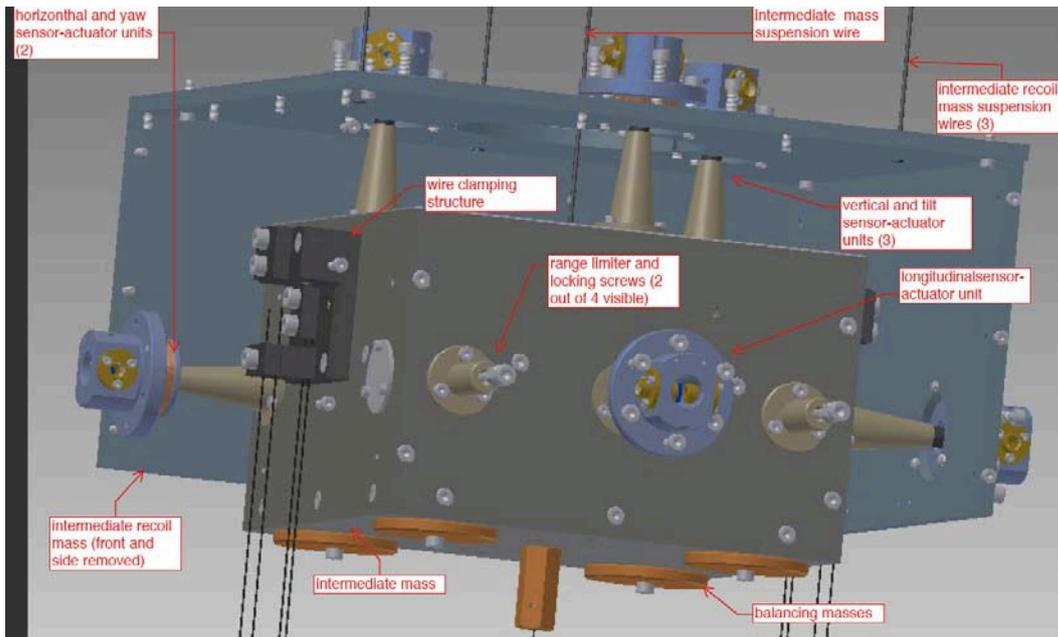
Figure 9: Illustration of the intermediate mass surrounded by its recoil mass. The front and side plate of the recoil mass have been removed to allow observation of the components and their functionalities.
