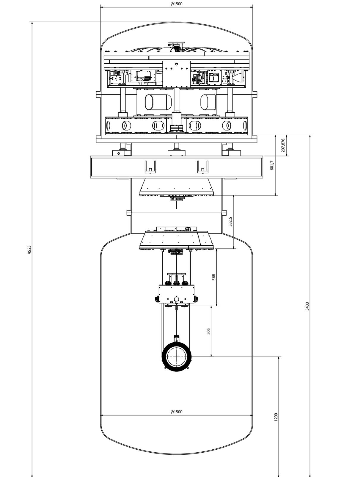
Figure 22: Two-D view of general assembly of the Type-B recycler seismic attenuation and suspension chain.
