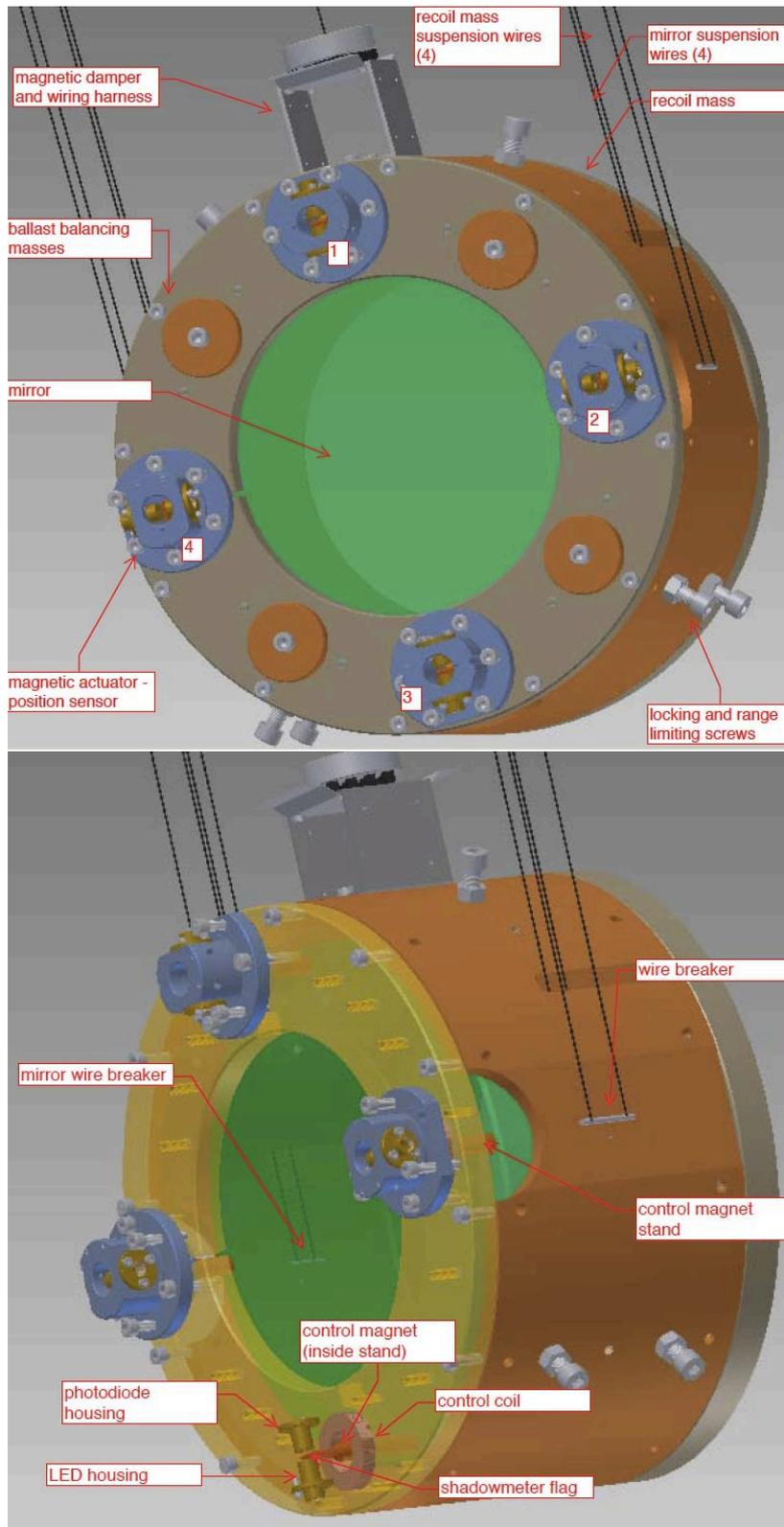
Figure 6: Recycler mirror mounted inside its recoil mass. In the lower image the back plate is made transparent and the body of one of the actuators have been removed for illustration purposes. The wires below the wire breakers are not shown.
