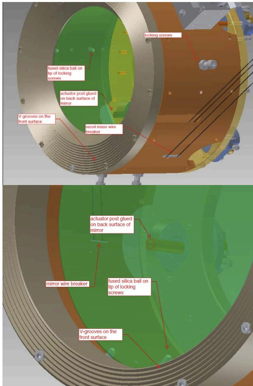
Figure 7: Top, front view of the PR2, PRM, SR2 and SRM mirrors. Bottom, front view of the PR1, and SR1 mirrors, with the wider clear aperture. In both cases the mirrors are imprisoned inside the recoil mass for safety.
