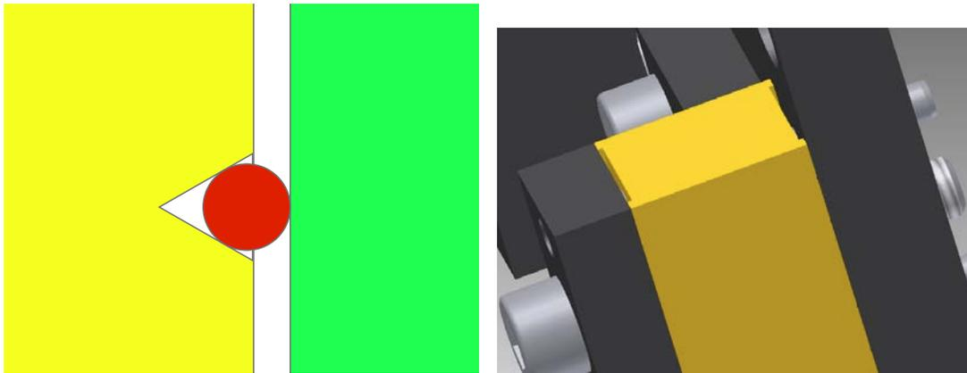
Figure 11: Illustration of positioning groove geometry with three-point 120° contact point on the clamp (left) and compression force concentration on clamp edge points (right).
