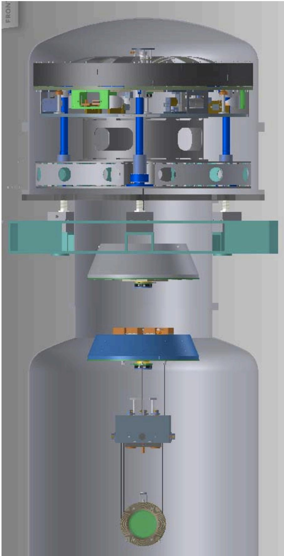
Figure 21: Three-D view of general assembly of the Type-B recycler seismic attenuation and suspension chain.
