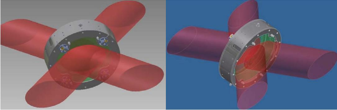
Figure 19: Illustration of the surface occupancy of 203 mm diameter beams on the front (reflective surface, top image) and back face (anti-reflective) of the beam splitter, and of the maximum allowable occupancy for the recoil mass and its instrumentation.
