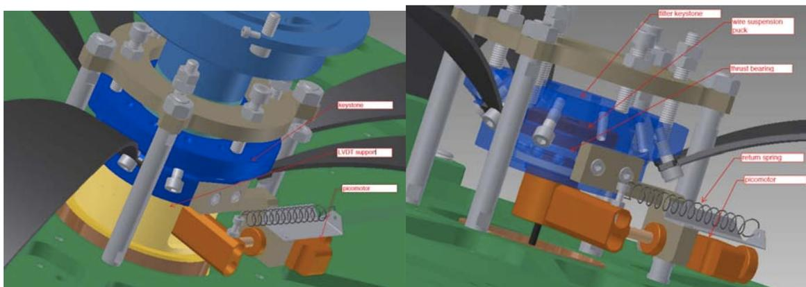
Figure 16 Rotation mechanism, Keystone made transparent on right panel.
