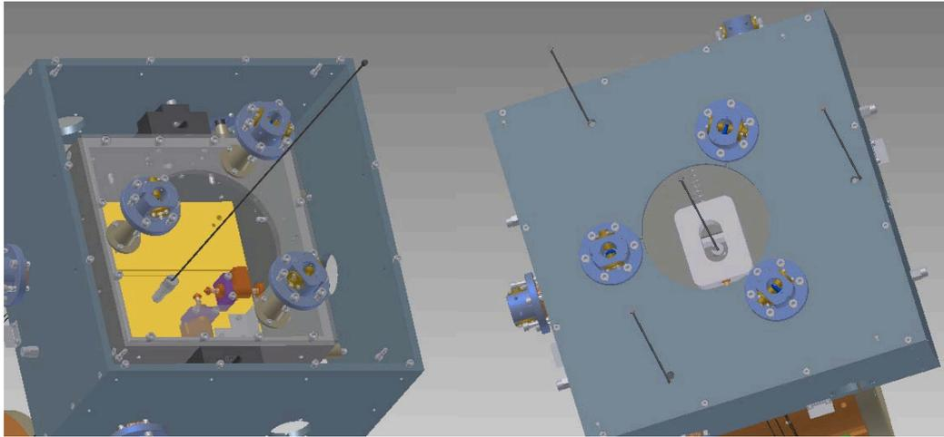
Figure 8: support point for the intermediate mass (left) and its recoil mass (right).
