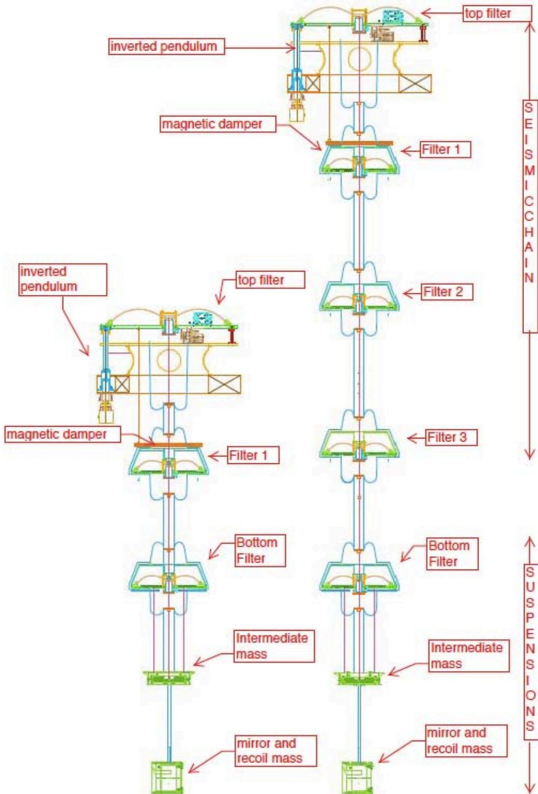
Figure1: Schematic, topological (not to scale) view of the seismic attenuation and mirror suspension chains. On the left: recycler or beam splitter mirror chains (type-B). On the right: test mass mirror chains (type-B). Most components are common to both chains. Only the intermediate mass and mirrors are different, and, of course, the spring's strength and the wire lengths and sizes.
