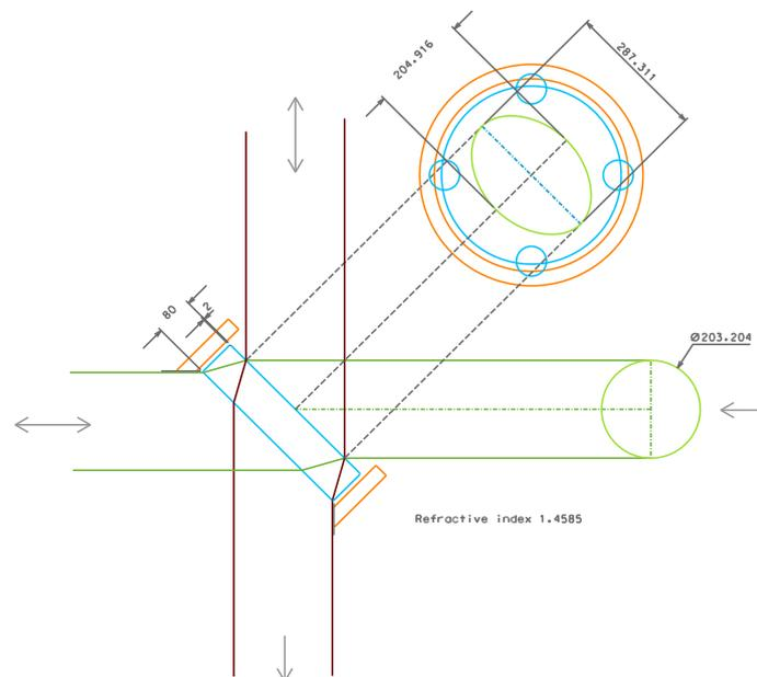
Figure 18: Scheme of the maximum circular clear aperture of the beam splitter. There is substantial free space for the actuators above and below the beam profile in the front face (50% reflectivity face).
