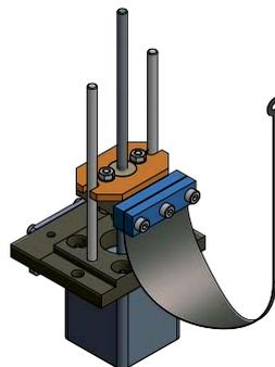
Figure 4: Close-up of the top filter vertical working point adjustment stepper motor mechanism. A stepper motor acting on a soft spring adjusts the vertical working point of the top filter and offloads any static vertical force requirement from the suspension dynamic actuators.
