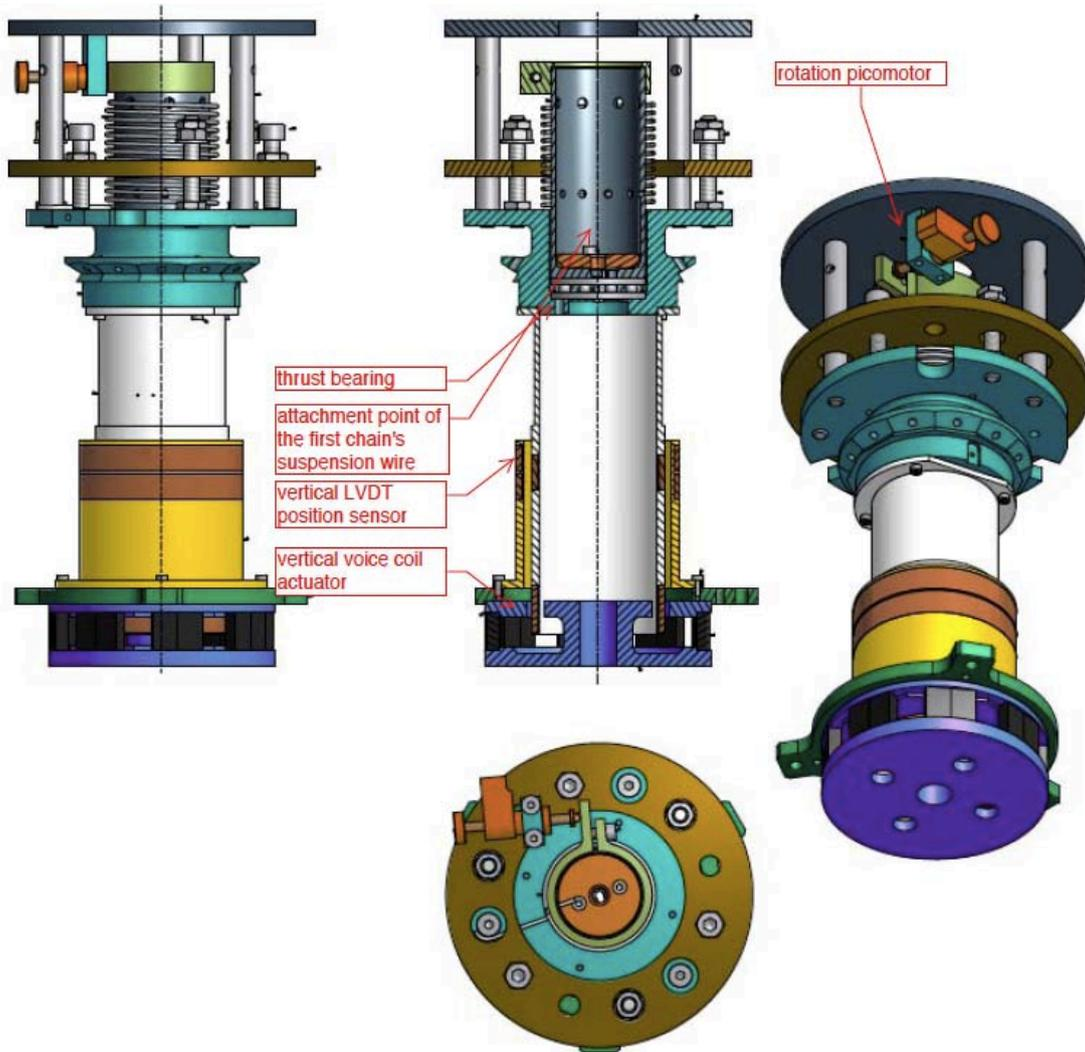
Figure 3: Close-up of the top filter suspension point rotational mechanism. A picomotor acting on a thrust bearing against a recoil springs can rotate the suspension point of the seismic chain and offloads any static yaw force requirement from the suspension dynamic actuators.
