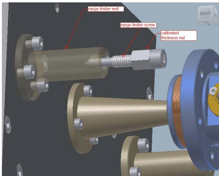
Figure 12: Illustration of the range limiters that keep accidental motion from damaging the magnetic actuators (the plate supporting the screw has been removed to allow view of the structure). When fully engaged the calibrated nuts of the range limiters lock the position of the intermediate mass at the exact center of its recoil mass.
