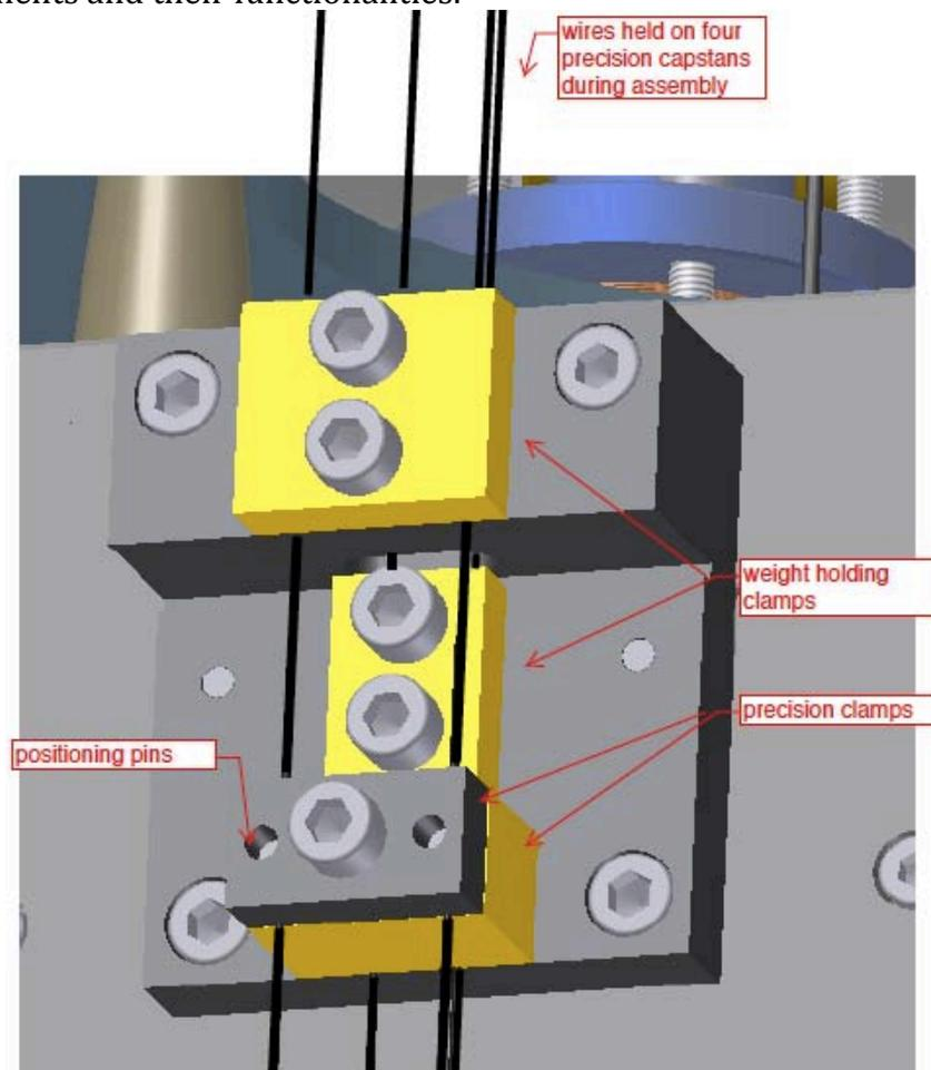
Figure 10: Illustration of the wire-clamping scheme with separate clamping for weight support and for pendulum flexure point definition.
