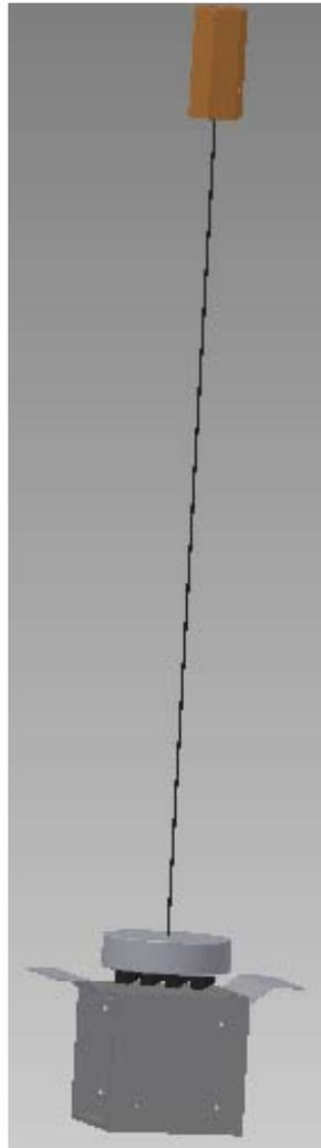
Figure 13: Whip extending from intermediate mass, carrying 4x4 damping magnets, hovering above damping plate on top of the mirror recoil mass. The gull wings are for electrical cabling.
