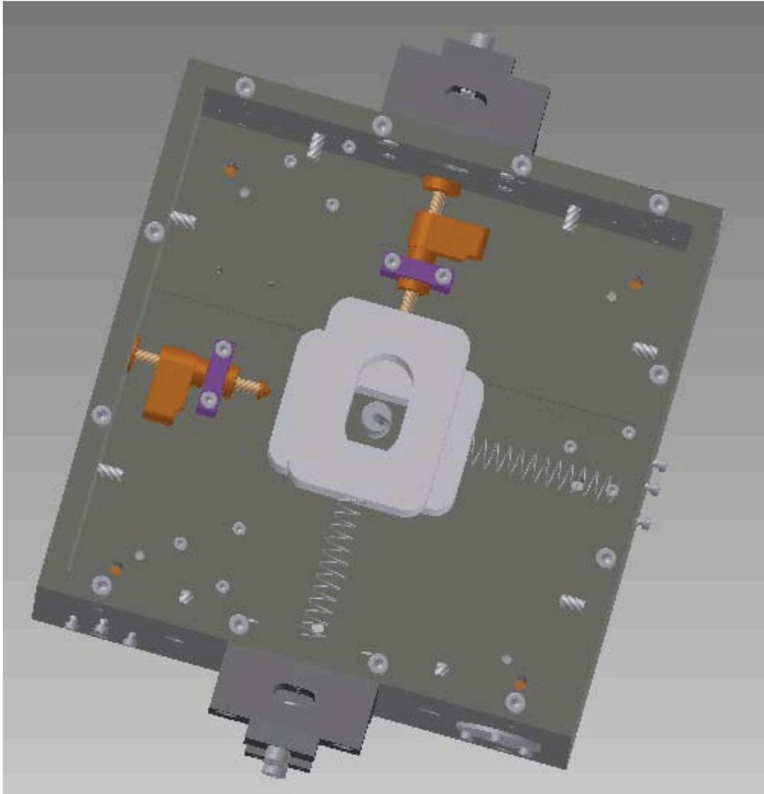
Figure 14: structure of the picomotor actuated balance masses. The cover plate and the guide plates have been removed to allow observation.
