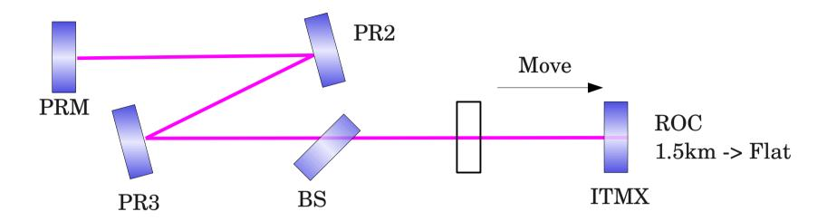
Need to tweak the positions and orientations of PR2, PR3 and BS to make the beam normal incidence to ITMs
