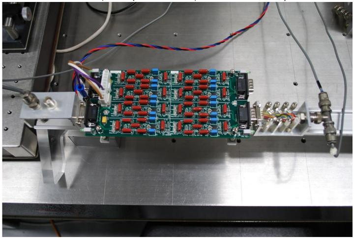
Fully-differential low-pass filter, 8 channels per a board
