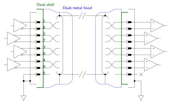
STP cable with D-sub connector
