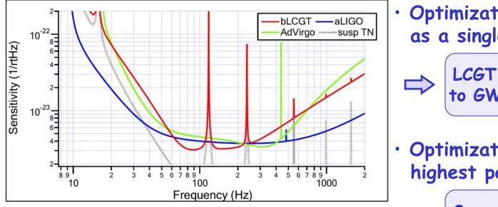
IR=309Mpc (aLIGO), 242Mpc (AdVirgo), 273Mpc (LCGT) \*Without suspension TN, IR of LCGT would be 301Mpc. • Optimization so far was for LCGT as a single detector
