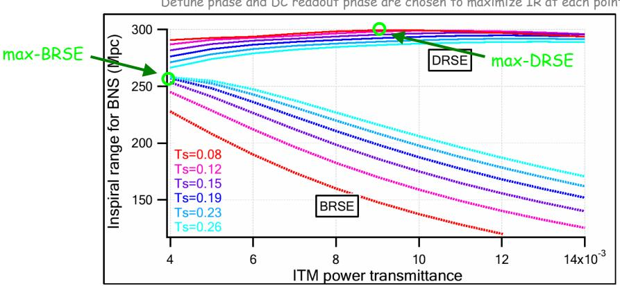
Detune phase and DC readout phase are chosen to maximize IR at each point
