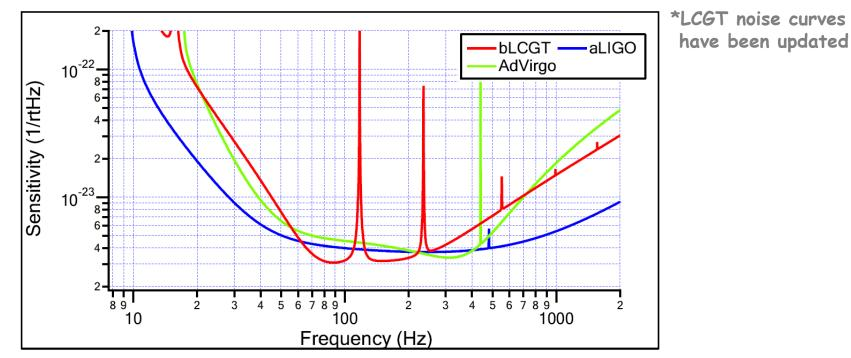
IR=309Mpc (aLIGO), 242Mpc (AdVirgo), 273Mpc (LCGT) [309Mpc x  $\frac{3}{4}$  =231Mpc]
