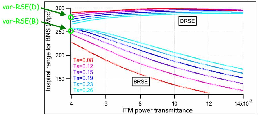
Variable-RSE with an intermediate optical setup
