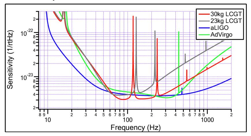
[parameters] 25cmLCGT: m=30kg, w=3.5/4.5cm, I=75W, Tm=20K 22cmLCGT: m=22.8kg, w=4.0/4.0cm, I=25W, Tm=20K
