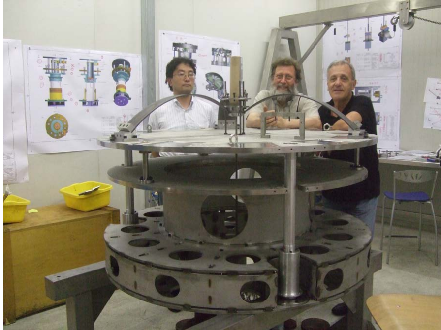
Figure 3: First assembly of the Top Filter unit. The blades of the Top filter lift about 100 kg each, they cannot be pulled by hand anymore. A special screw driven tool was designed.
