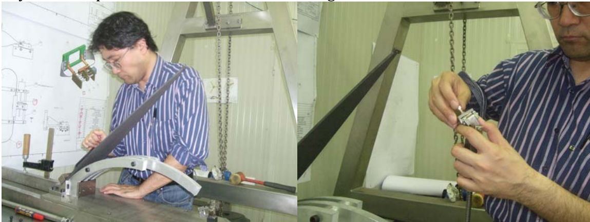
Figure 3: First assembly of the Top Filter unit. The blades of the Top filter lift about 100 kg each, they cannot be pulled by hand anymore. A special screw driven tool was designed.
