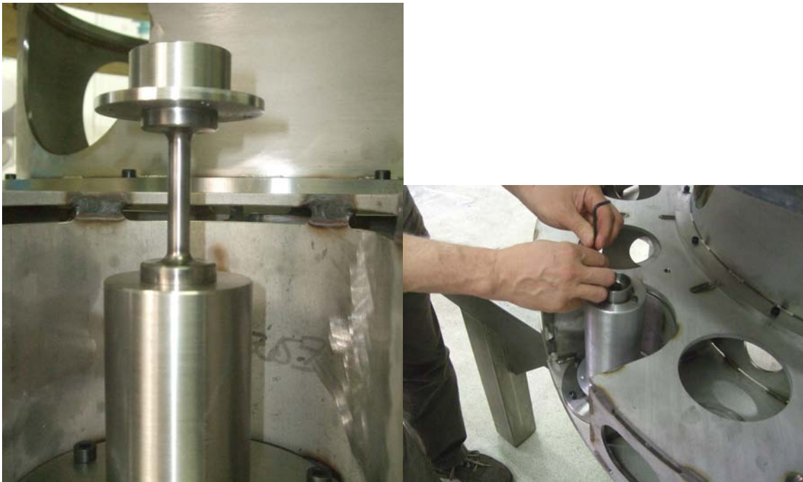
Figure 5L : The tuning masses are 120^\circ arches with 40 mm 20 mm, 10 mm and 5 mm thickness, that can be bolted on the outer rim of the filter to form whatever load mass necessary to tune the Inverted pendulum at the desired frequency. Figure 5R: Cable passage slot to bring the cables to the sensors and actuators operating on the top filter.
