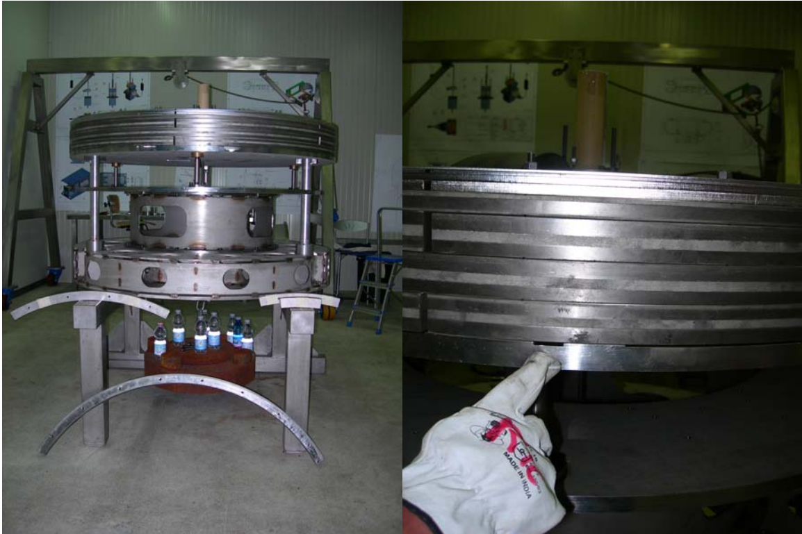
Figure 5L : The tuning masses are 120^\circ arches with 40 mm 20 mm, 10 mm and 5 mm thickness, that can be bolted on the outer rim of the filter to form whatever load mass necessary to tune the Inverted pendulum at the desired frequency. Figure 5R: Cable passage slot to bring the cables to the sensors and actuators operating on the top filter.
