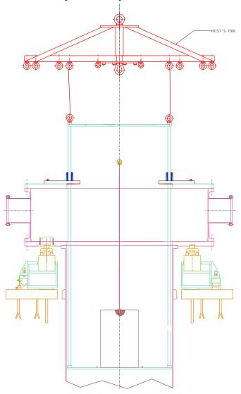
The filter number 3 is craned in, sat over the safety harness, connected to the ballast mass temporary wire using the wire connection box. The lower wiring spider of filter 3 has to be in position already.
