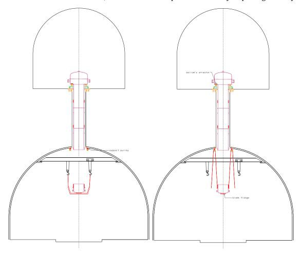
All viewports are sealed. The chamber is connected to a vacuum pumping unit. When the vacuum assembly is closed it is UHV tested for leaks, to make sure that all unreachable flanges are perfectly sealed. Plastic foil lining taped to the cylindrical surface of the spools, and thin plastic tubes allow blowing Helium around each unreachable flange, to identify location of possible leaks.
