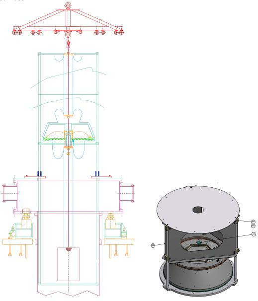
Filter 3 is lowered on pads sitting on its safety ring. The pads keep it lifted by several cm, so that its suspension wire sticks out sufficiently above the safety ring of filter 2 to be easily attached to filter 2.
