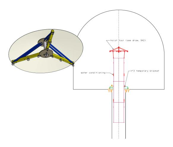
When all the spools are in place, the top chamber "bath tub" is installed.
