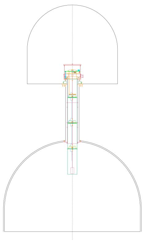
The unit Top filter and Inverted Pendulum is lowered in place, but is still disconnected from filter 1.
