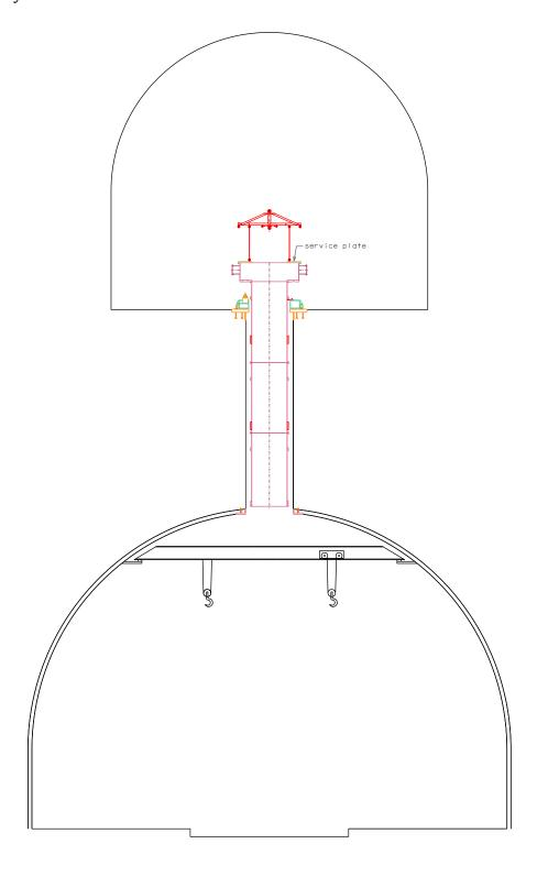
The top dome is mounted on the tub, the lower dome is raised by means of the two cranes of the lower chamber so that it can be hooked to manual chain hoists, and connected to the lower spool.
