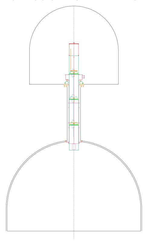
The safety structure between the Top filter and filter 3 is assembled, as well as the suspension wire of filter 3, electrical wiring, and its Eddy current damping ring.
