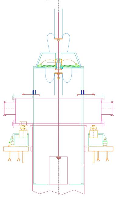
The safety structure between filter 3 and filter 2 is built, and stiffened with two pairs of three temporary panels, as shown in the side figure.
