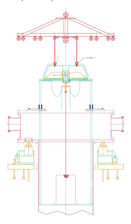
The filter 3 suspension wire, and its spiders are mounted. Cabling is done around filter 3 and between its lower and upper spiders.
