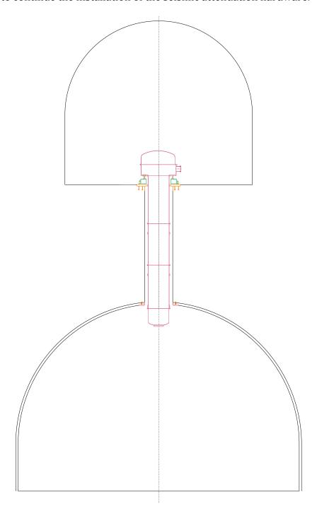
The ballast mass ( $\sim$ 300 kg, precisely adjusted to the lift load of filter 3 at 21°C) is lowered over a temporary safety disk, a temporary safety structure is built, the ballast temporary suspension wire is mounted.
