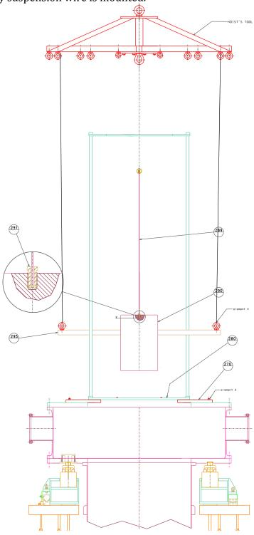
The temporary ballast safety structure is lowered in the well  $\frac{3}{4}$  way, and fastened with three safety conical clamps to the top of the tub.
