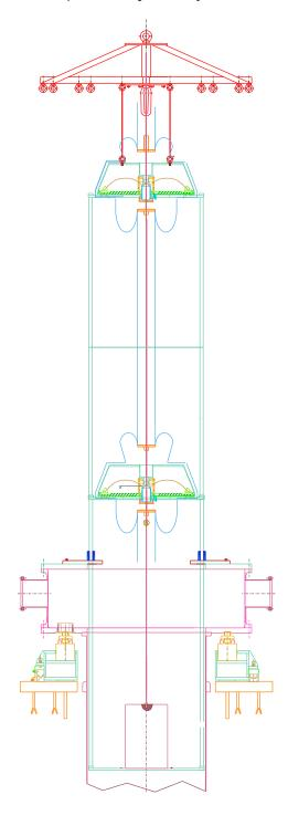
Filter 2 and 3 are lowered on their safety rings, the safety structure is lifted, the conical clamps are removed so that the structure can be lowered by one step and reclamped.
