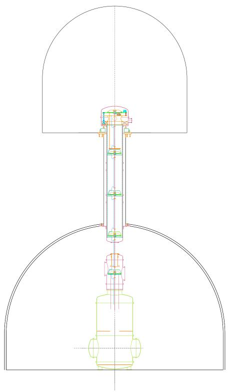
The vacuum chambers are positioned (note only the top, pink, part needs to be removed to insert the SAS chain). Filter 4 is inserted on a stretcher, connected at the junction box and electrically wired. Then the vacuum neck above is closed.
