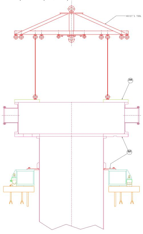
The hydraulic jacks supporting the vacuum chamber and the Inverted pendulum are positioned in the sled, the Inverted pendulum bellows are installed, and the vacuum assembly is lowered on its stand.
