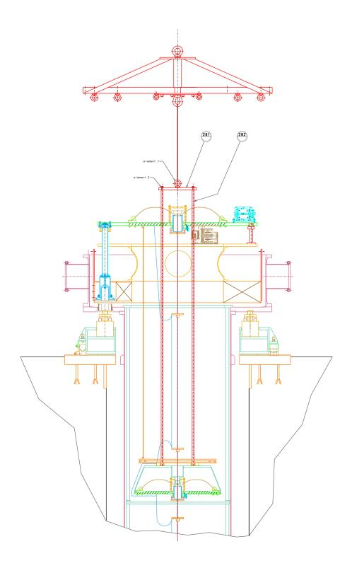
Special lifting rods are inserted through holes into the top filter, are screwed into the roof of filter 1, and used to lift it, so that its wires can be attached to filter zero. The functionalities of all filters are re-checked.
