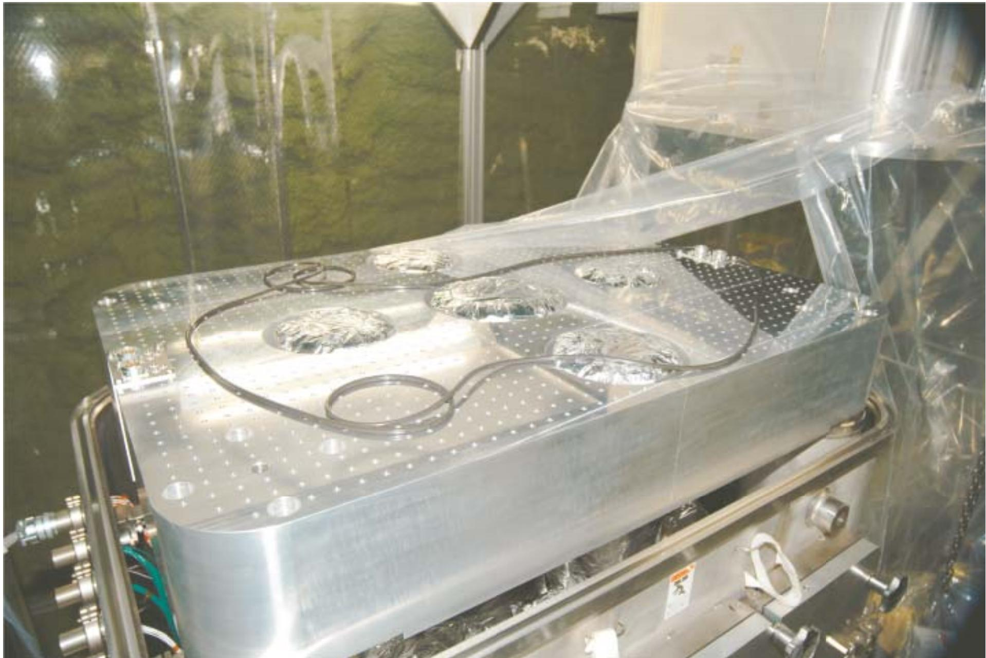
Cryostat of CLIO interferometer
