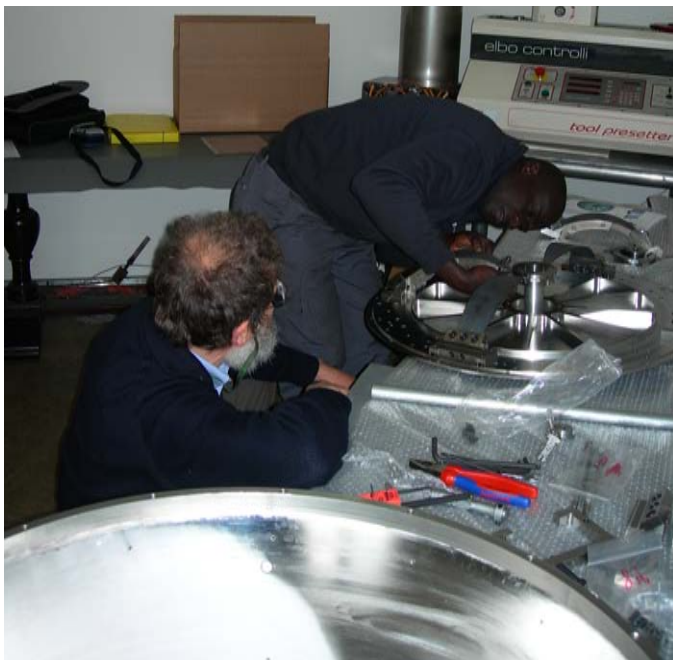
Figure 11: Top to bottom, presenting the pre-stressed blade into the keystone, which is held in place by the holding column, note in the second image the small angle between the blade's tip and the keystone, that will disappear as the blade is released, two opposite blades are mounted at the same time to null transverse stress., the blade is tied to the keystone with a retaining screw.
