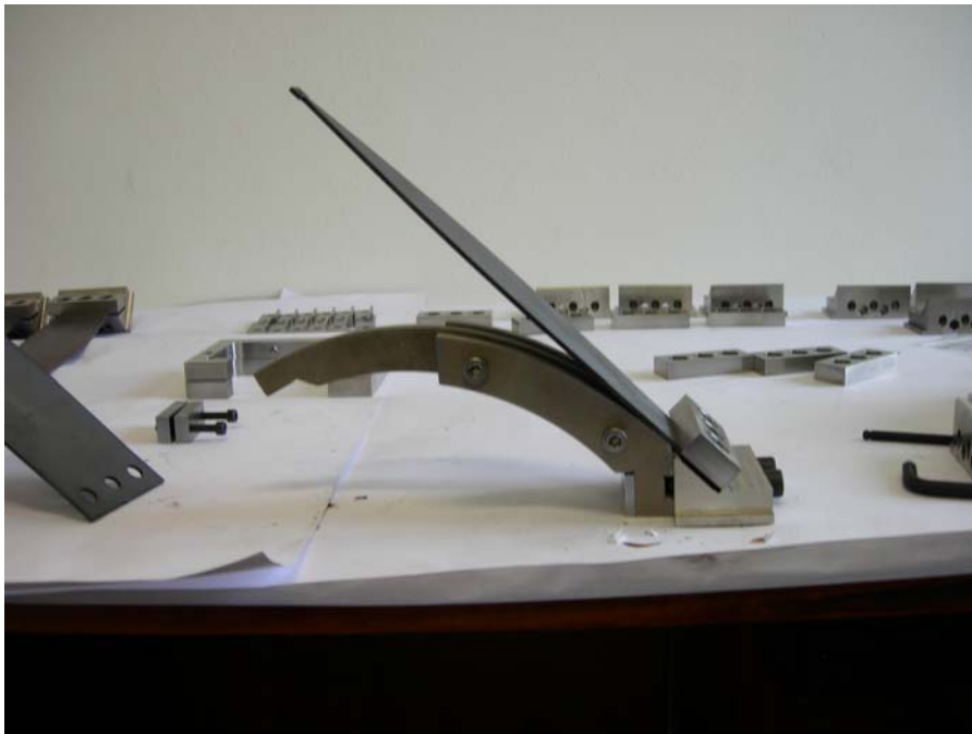
Figure 4: Above, blades, blade clamp with pre-stressing transport arch, and a blade with the bending pulling handle with homo-kinetic joint. Below blade clamped with transport arch bolted to the blade clamp.
