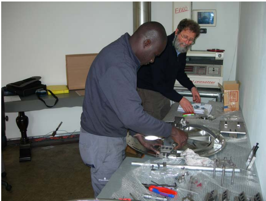
Figure 12: Top, the holder clamp is removed from the tip of the two opposite blades. Bottom, The bending arch is released from the blade clamp and removed. The blade's tip holding screw is then tightened.
