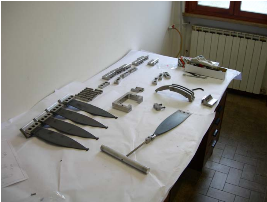
Figure 3: Standard filter parts ready for assembly: Top: base plate with keystone holding tool, Bottom blades in clamp. Frequency tuning horseshoe, blade with pulling tool, bending arch and clamps.
