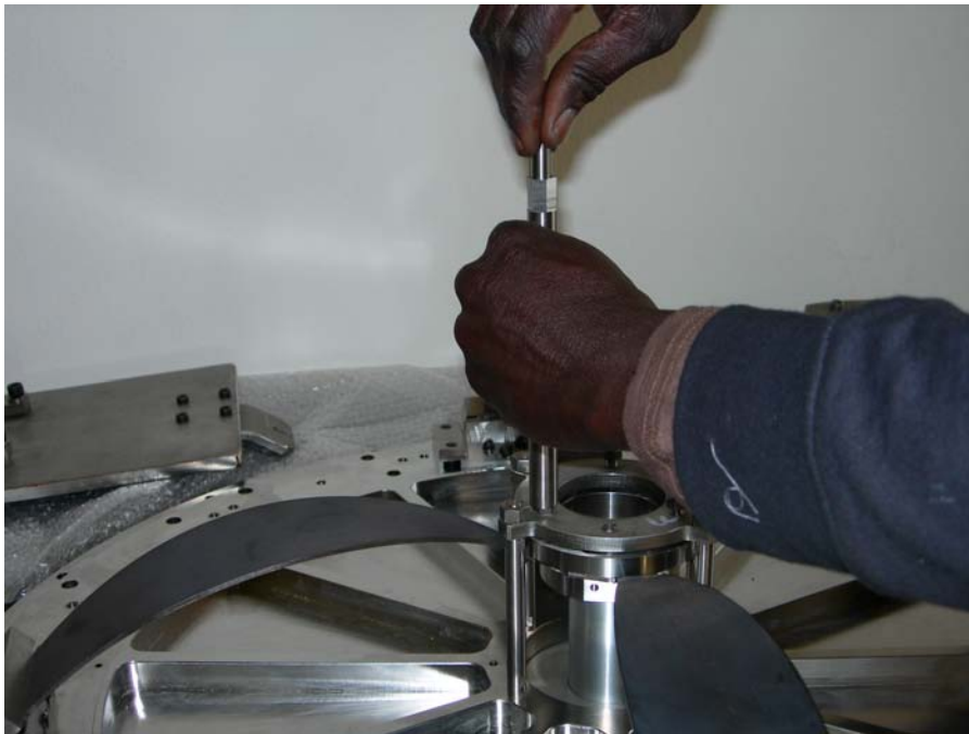
Figure 14: The stress is transferred to the keystone end stop ring and locked at the desired height using the custom coaxial tool.
