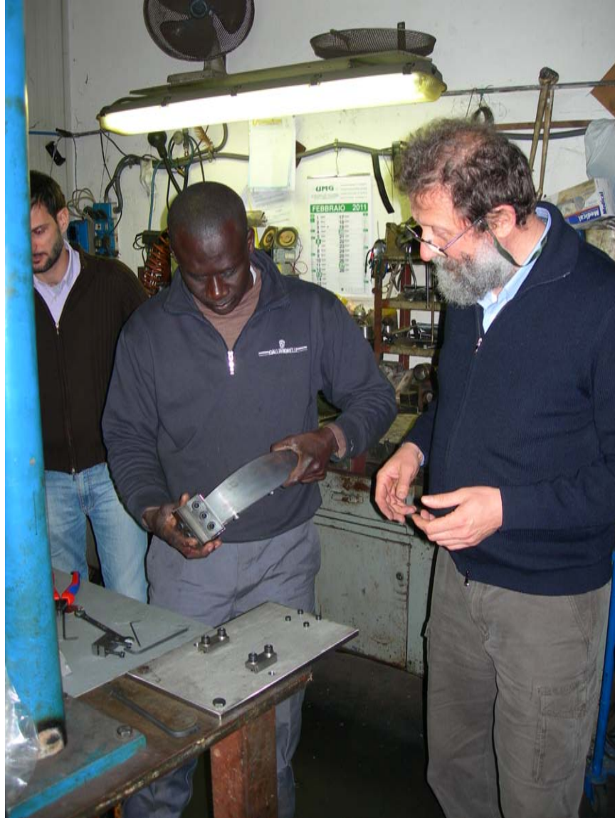
Figure 10: Removing the pre-stressed blade from bending fixture.
