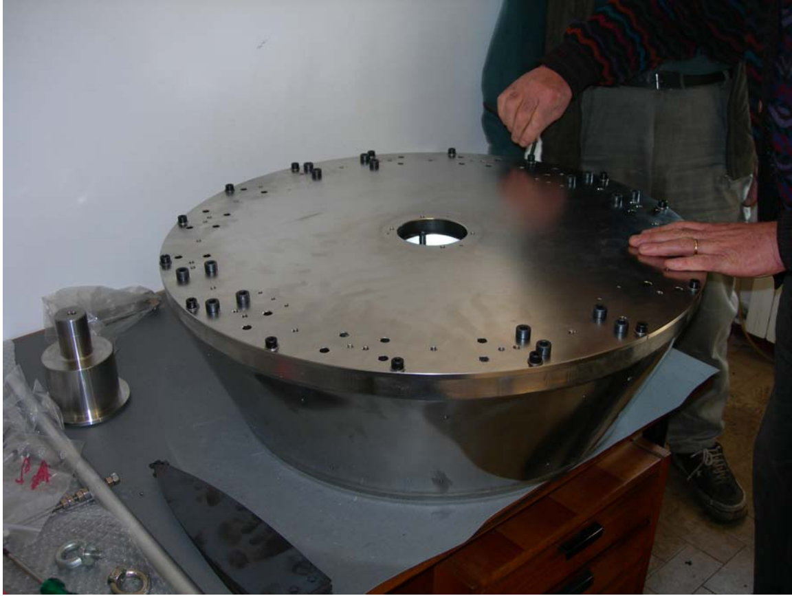
Figure 17: Top to bottom, the wire suspension nose is mounted in the filter shell, the filter mounted inside the shell and bolted closed.
