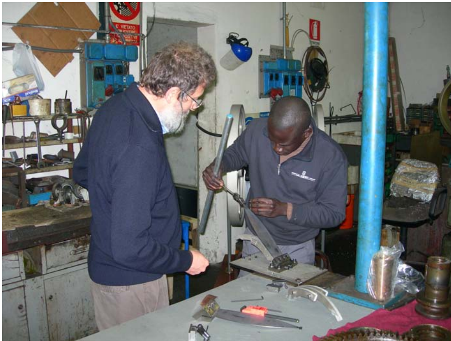
Figure 6: Top, relaxed blade and bending arch being mounted on blade's clamp. Bottom pulling handle being mounted on tip of blade. Tanzir Fall Madieye is performing the assembly, he is the proposed chief of assembly, he has already assisted the clean assembly of the HAM SAS for LIGO.
