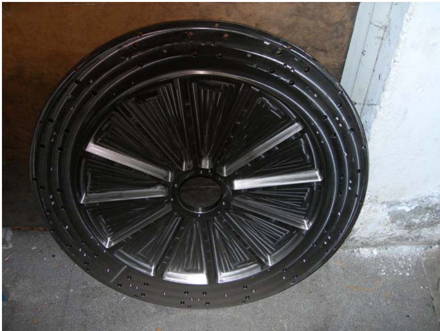
Figure 1: Machining of the standard filter base plate with water-soluble coolant/lubricant, and the finished product.
