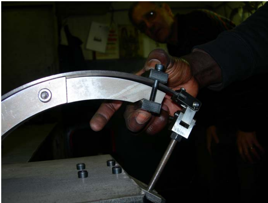
Figure 7: Top, pre-stressing the blade and hooking the pulling handle to its stop. Bottom transferring the load to a holding fixture.
