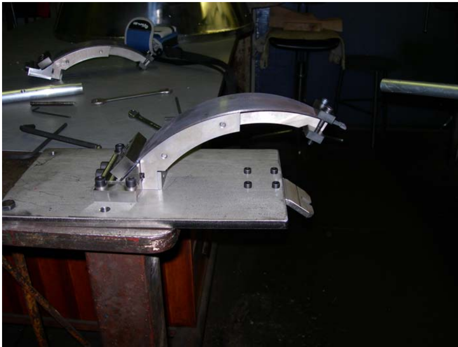
Figure 8: Top to bottom, mounting and tightening the holding fixture, removing the pulling handle, pre-stressed blade ready for installation.
