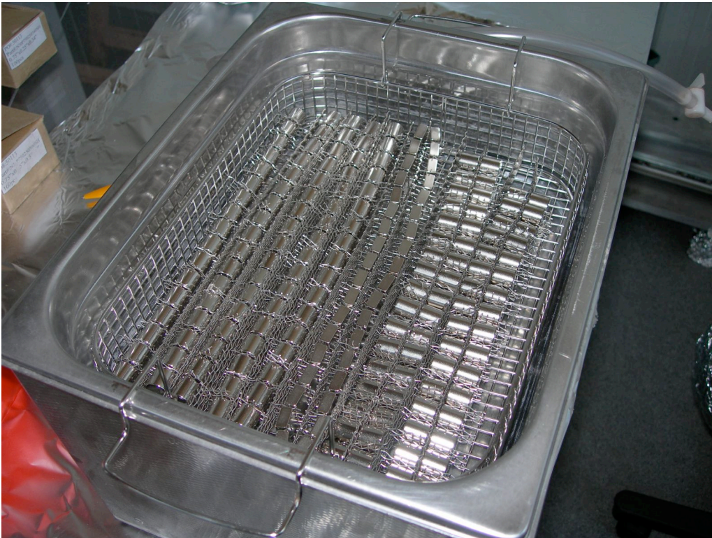
Parasitic tuning spring motorized sleds are assembled and baked
