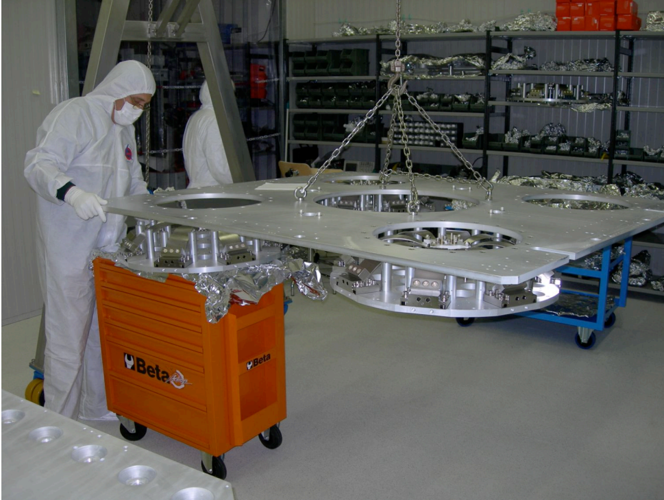
Mounting the GAS filters in the spring box. A second aluminum plate will then complete the box and give it its rigidity.
