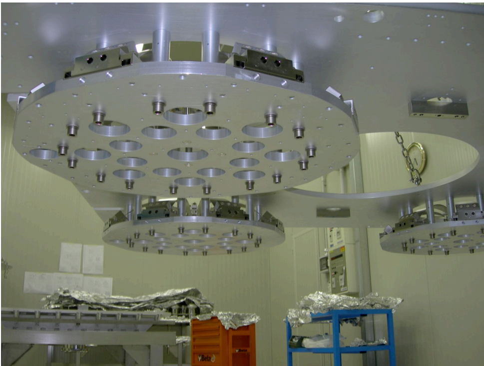
Mounting the GAS filters in the spring box. A second aluminum plate will then complete the box and give it its rigidity.
