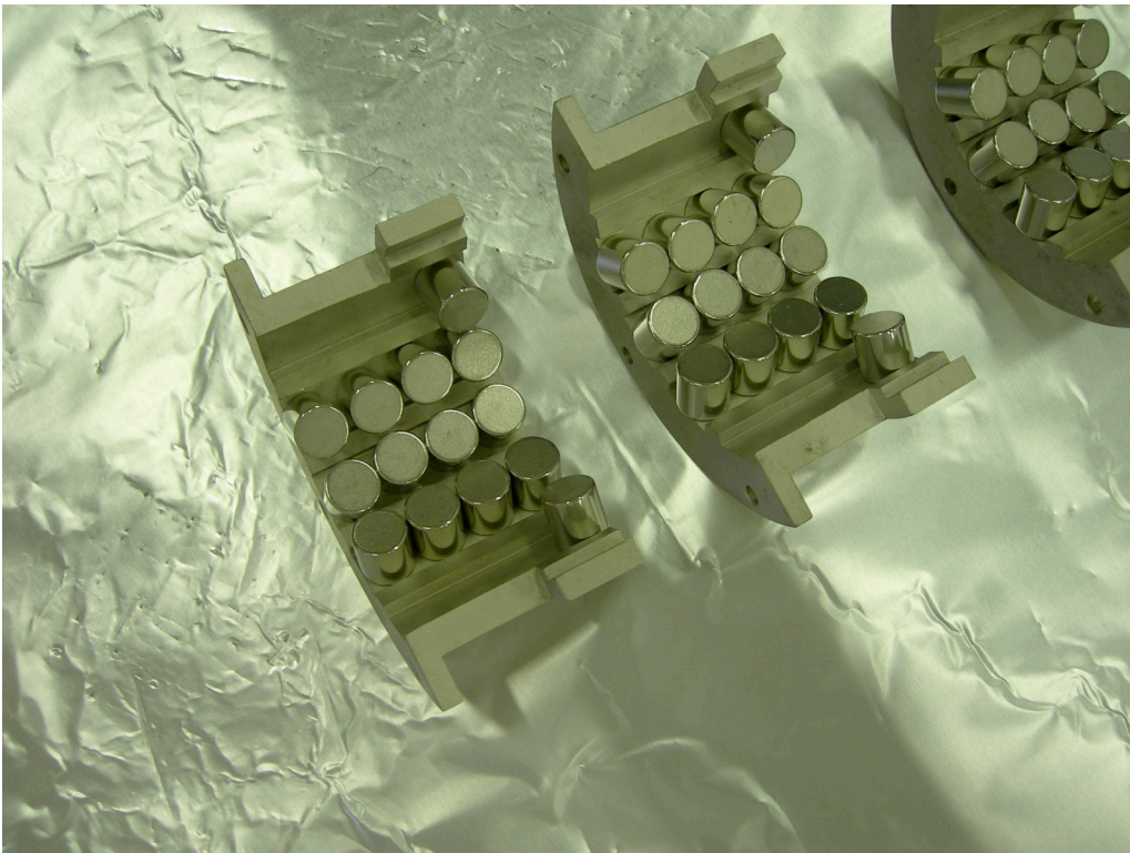
Magnetic dampers eliminating the leg rigid body first resonance.
