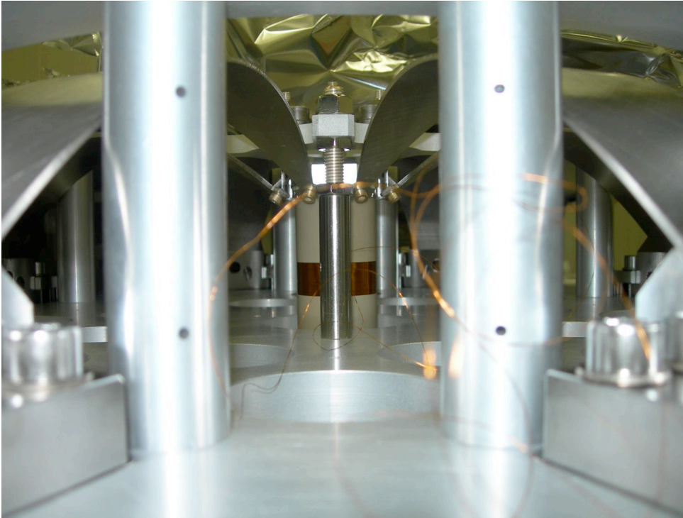
The LVDT primary and actuator coil cylinder is mounted on a GAS filter Key-stone .
