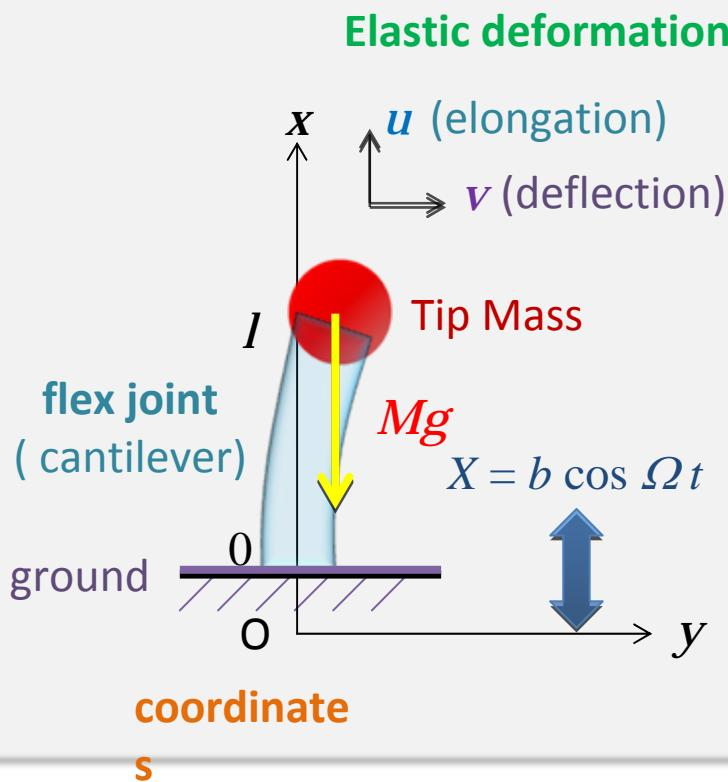
Flex joint was modelled in a continuous system as an elastic body.
