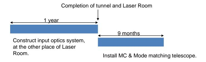
Before completion of tunnel and Laser Room, construct the input optics system include pre-MC and ref-Cav with high power laser at the other place of the Laser Room.
