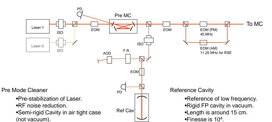
•Cavity pole is around 300 kHz.
