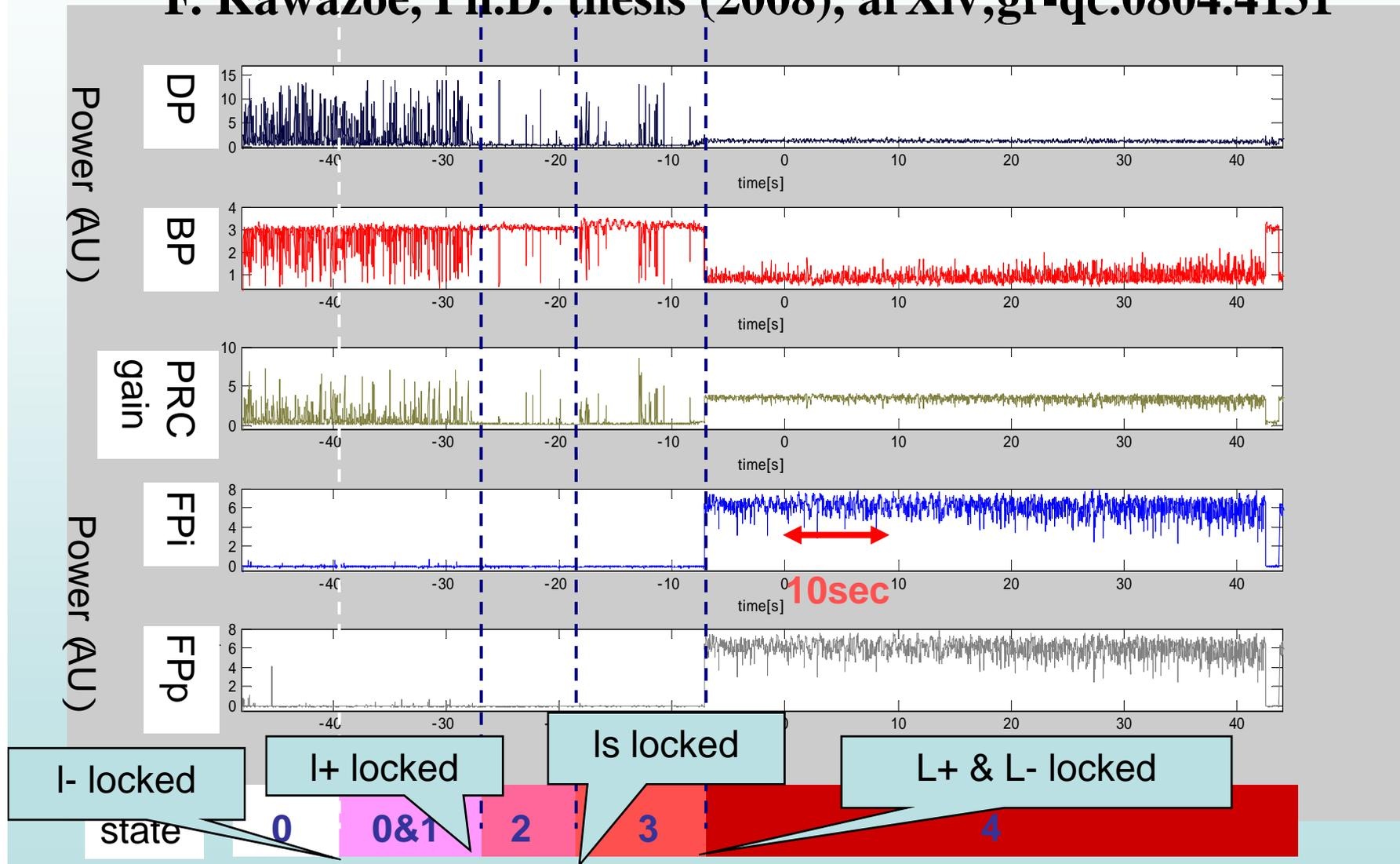
0: not controlled    1: I- locked    2: I-, I+ locked    3: I-, I+, Is (central part) locked
