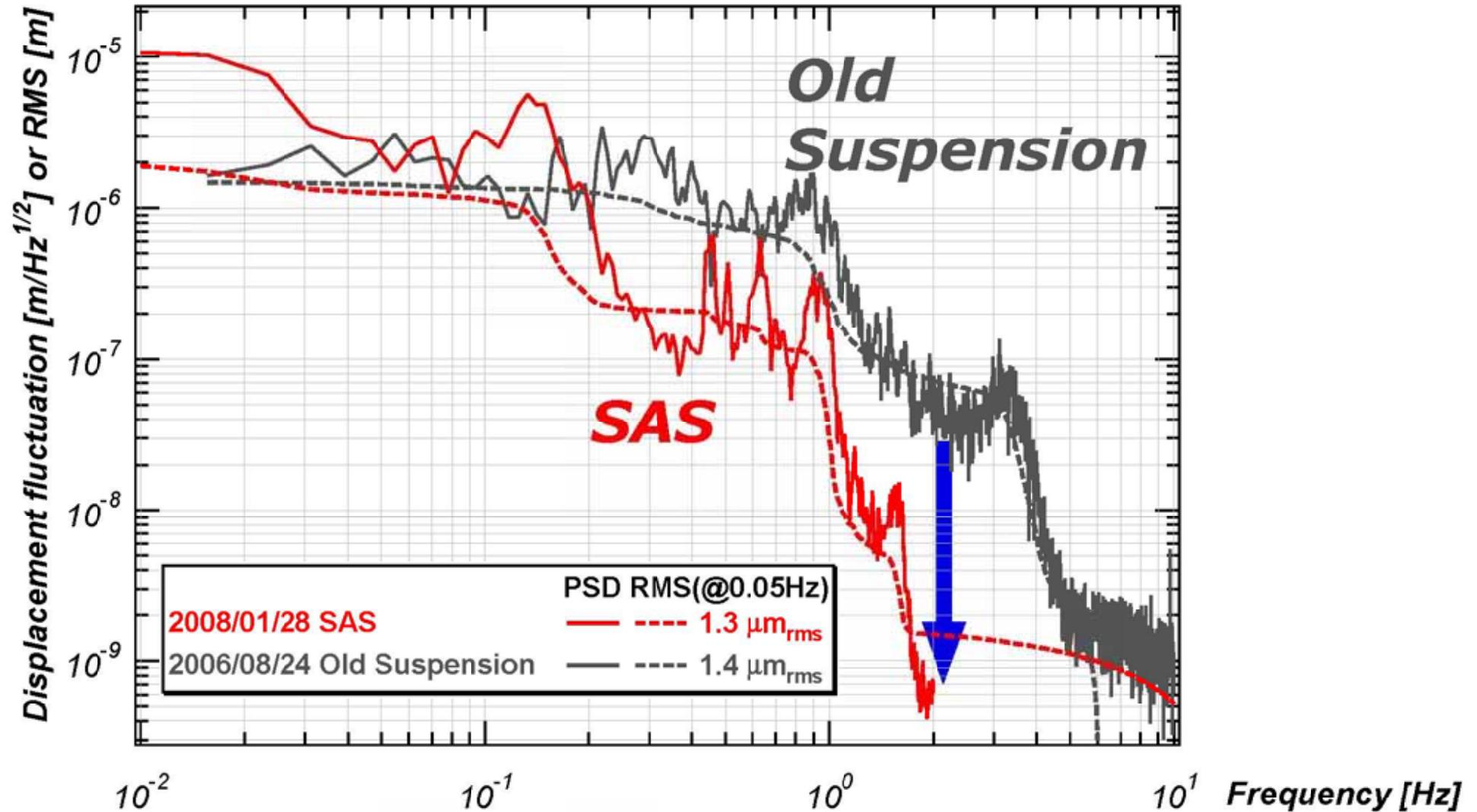
**10 times smaller** seismic noise **above 0.2 Hz**
