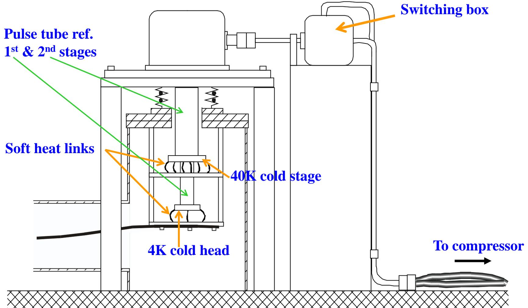
We **measured vibration** caused by **new** cryocoolers in **Kamioka** mine !
