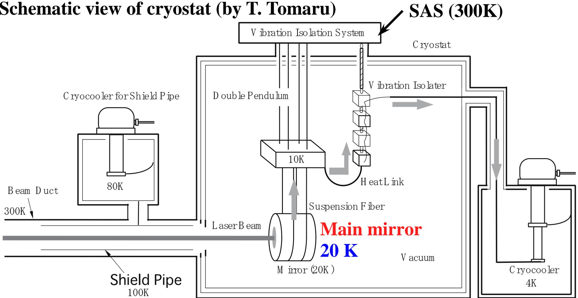
**CLIO** cryostat have already been **installed**
